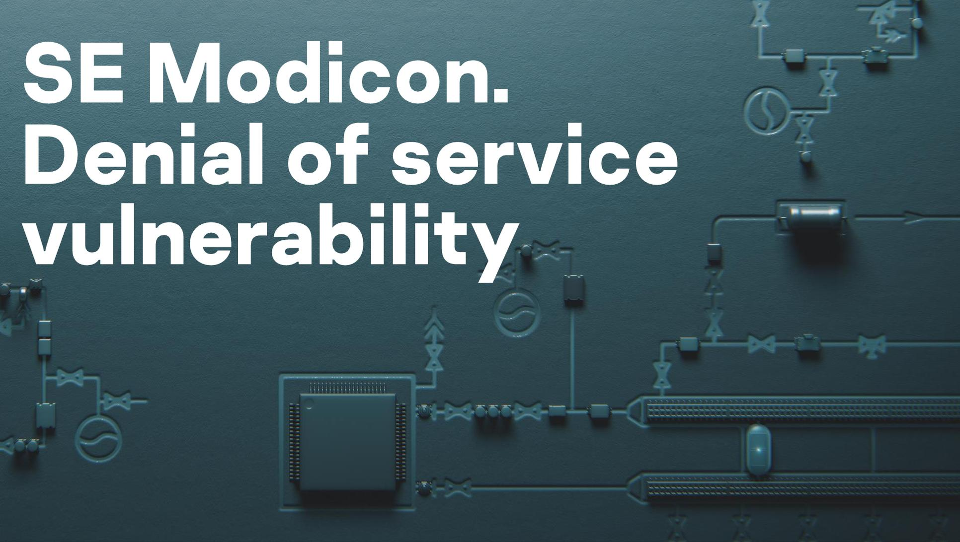
**“ A CWE-248 Uncaught Exception vulnerability exists which could cause a denial of service when sending invalid debug parameters to the controller over Modbus.**
