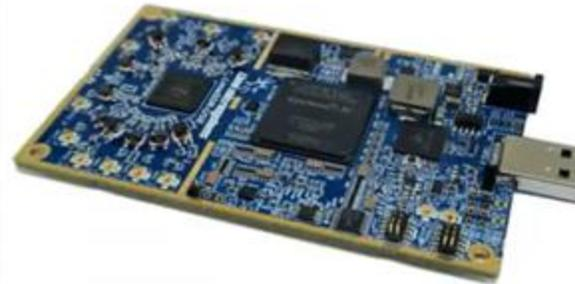
LimeSDR Flexible, Next-generation, Open Source Software Defined Radio USB 3.0 100 kHz - 3.8 GHz
