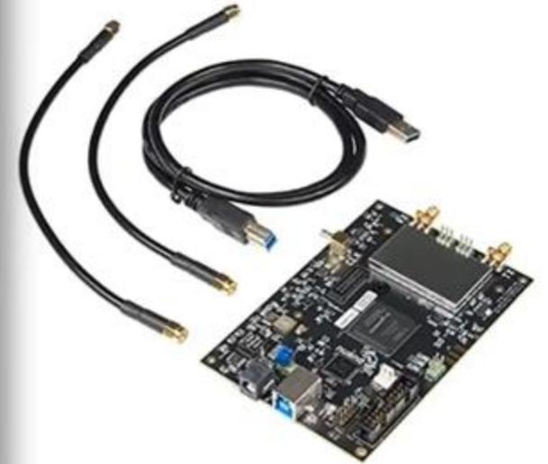
bladeRF 2.0 micro xA4, 47MHz to 6GHz frequency range, 61.44MHz sampling rate, 2x2 MIMO channels USB 3.0 SuperSpeed Software Defined Radio.
