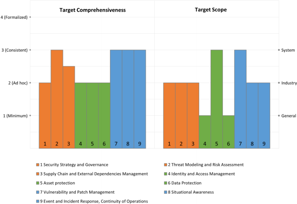
Smart Bottling Line Security Maturity Target: Determining needs and setting out the initial comprehensiveness and scope for subdomains
